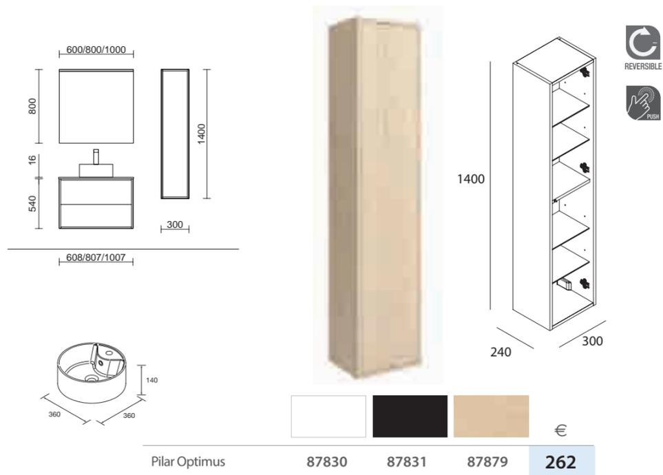
Technical drawing showing dimensions: 600/800/1000 (width), 800 (height), 16 (thickness), 540 (height to top), 300 (depth), 1400 (height), 240 (width), 300 (depth). Includes icons for REVERSIBLE and PUSH. A circular detail shows a 360-degree rotation.
